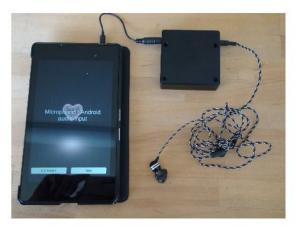
Detected and processed vital signal from earphone is sent to smartphone or PC through mic terminal of earphone jack. It's possible to install all in PC or smartphone if we can rework inside . The adapter with display software written in Unity environment is able to apply to different types of OS on smartphone or PC .
