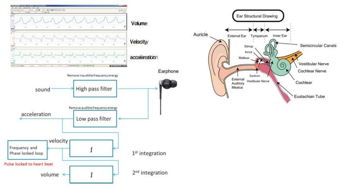
The principle is the frequency division multiplex. With it, it becomes possible to use an earphone as speaker in audible frequency band and as a microphone in inaudible lower frequency band.
